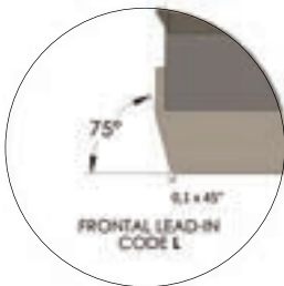
"L" lead-in to reduce the feed of 40% compared with the values on pages 8-9
