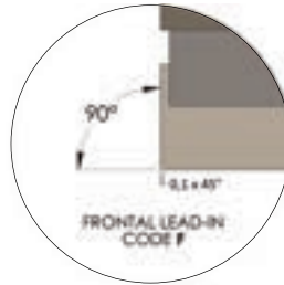
"F" lead-in to reduce the feed of 40% compared with the values on pages 8-9
